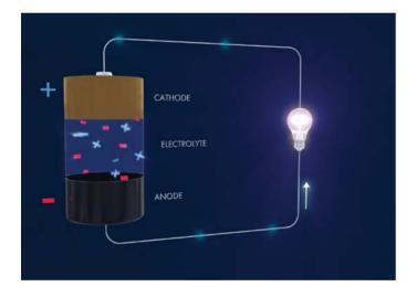
For an illustration of past technologies, the image to the left shows a simple circuit with a load - a battery illuminating a light bulb. For a battery to work properly, a molecule needs to act as an electron donor- a reducing agent. In the example above, this is the black anode, which is shown as negative because of the abundance of negatively charged electrons it provides.
